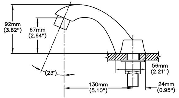
INLETS: 1/2" MIP/COUPLING NUTS (NUTS NOT SUPPLIED)
