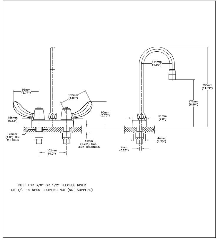
Delta reserves the right (1) to make changes to specifications and materials, and (2) to change or discontinue models, both without notice or obligation. Dimensions are for reference. Measurement may vary plus or minus 6mm(0.25"). Mounting locations are suggested only. Check with local codes for requirements in your area. This spec was produced April 22, 2021.
