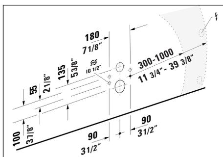
Set the height of the toilet based on the position of the drain according to the technical drawing of the toilet.
