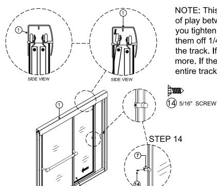
STEP 14 Attach the knob to the end of the inside panel that is furthest from the shower head.
