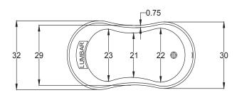
OVERFLOW IS INTEGRAL TO THE TUB
