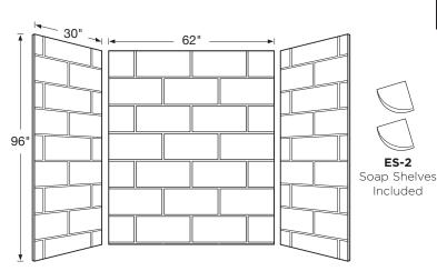
Designed to fit base areas 30" deep or smaller x 62" wide x 96" high or smaller (762 mm x 1575 mm x 2438 mm)
