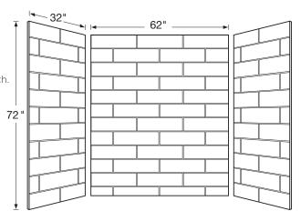
Designed to fit base areas 32" deep or smaller x 62" wide x 72" high or smaller (813 mm x 1575 mm x 1829 mm)
