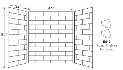
Designed to fit base areas 32" deep or smaller x 62" wide x 96" high or smaller (813 mm x 1575 mm x 2438 mm)
